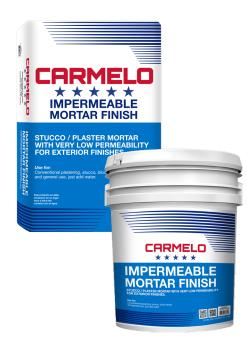
**Product Description:** Our IMPERMEABLE MORTAR FINISH is a blend of cement, especially graded masonry sand, and admixtures combined in carefully controlled proportions. The mortar was designed specifically for reducing the chance of water entering through the finishes on existing structures. It also provides a damp-proof finish that combines an easy-to-use formula, needing only water and with excellent performance.
